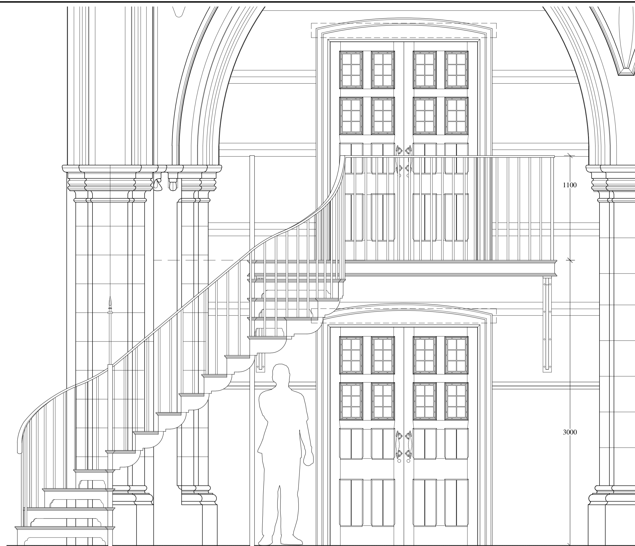
02 Proposed Steps Elevation B 1:20@A1
